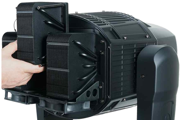
6. Unclip the center heatsink module safety cable.
